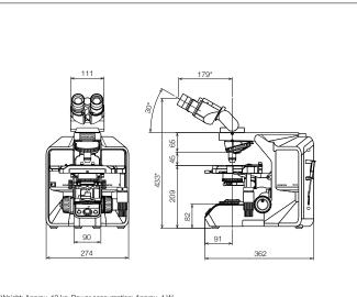
Weight: Approx. 21 kg, Power consumption: Approx. 330 W The length marked with an asterisk (\*) may vary according to interpupillary distance. Distance for figure shown is 62 mm.
